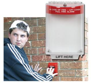
STI's protective polycarbonate covers, like the Universal Stopper<sup>®</sup> pictured in the upper right corner of this photo, fit over manual pull stations and have helped stop false fire alarms without restricting legitimate ones. When the cover is lifted to gain access to the actual pull station, a piercing warning horn sounds.
